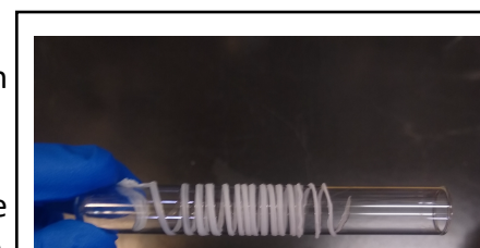
Image 2: An example of coiling the nylon around a test tube in Step 5.
