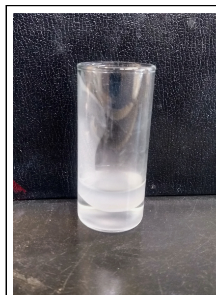
Image 1: An example of the two immiscible layers in Step 4 with the aqueous layer on bottom and organic layer on top
